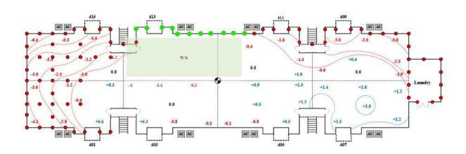
Green dots indicate locations of current major shifting units 413 and 411. Red dots indicate approximate locations of existing piles.
