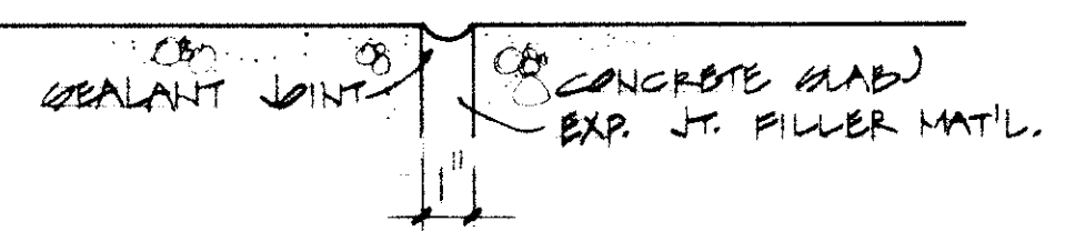
4 expansion joint thru balcony walk
